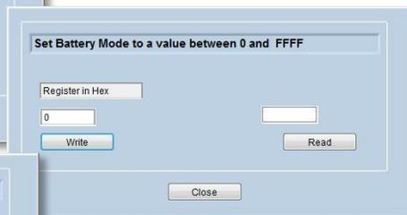
The **Battery Mode** feature can be used to select the various operational modes for the battery; for example whether the battery capacity is reported in mAh or mWh etc..
