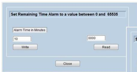
Similarly the **Remaining Time Alarm** can be adjusted to suit the length of time your users require to save their work and shut down the device. The default is set to 10 minutes on all Inspired Energy products.
