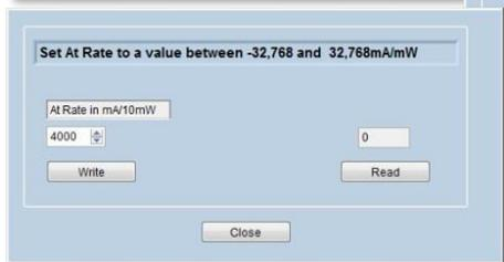
The "**AT-Rate**" function allows you to ask the battery questions. Literally "If I were to charge / discharge the battery **AT** the following **RATE**, how long will it take until the battery is full / empty?" Enter a negative integer for a discharge current and a positive integer for a charge current. **Note:** if you have used the battery Mode feature to change the capacity reporting from mAh to mWh you'll need to enter a value in mWh.
