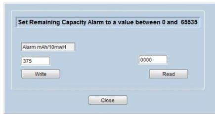
The **Remaining Capacity Alarm** can be altered to suit the needs of your device. By default, all Inspired Energy products have this value set to 10% of the design capacity. Open this window & enter a value to a value that will enable your device to shutdown "write button. The "Read" button
