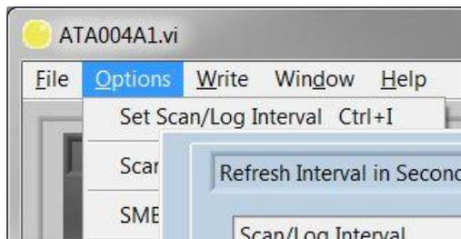
The **Scan / Log Interval** can be adjusted using this tab. Entering a value in seconds will change the scanning / data logging rate accordingly
